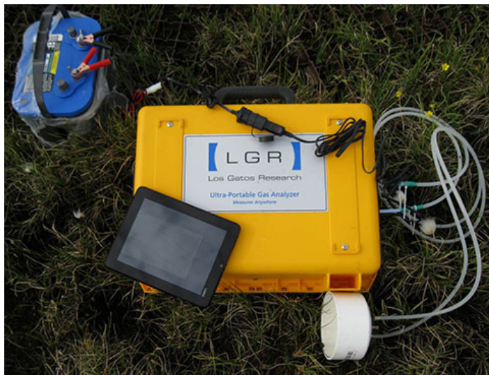
LGR's Ultra-Portable Greenhouse Gas Analyzer records methane, carbon dioxide and water vapor in real time in soil collars/chambers above the Arctic Circle (71° 15' N, 156° 37' W)
