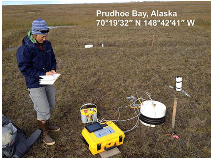
Ultra-Portable Greenhouse Gas Analyzer provides continuous measurements of CH 4 , CO 2 and H 2 O in soil chambers at Prudhoe Bay, Alaska, 70°19'32" N 148°42'41" W using only battery power (photo by United States Geological Survey)
